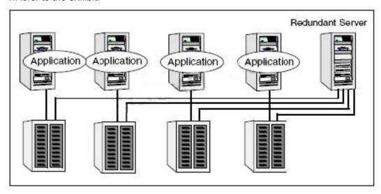
The exhibit shows an N-to-1 cluster configuration, in which nodes are connected to storage devices via dual-hosted SCSI cables.
