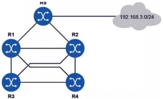
All routers in the diagram are running an interior gateway protocol (IGP) and have been configured with an ECMP value of 4. Router R5 advertises the prefix 192.168.3.0/24 using the IGP.
