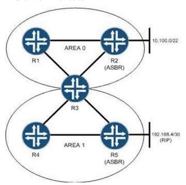
You are asked to configure an OSPF network based on the topology shown in the exhibit. You must keep the link-state database in Area 1 as small as possible. What will accomplish this?
