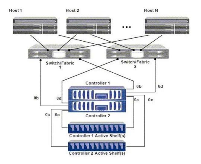
In the diagram shown, a portset is created on controller 1 with the command: controller1>portset create -f
